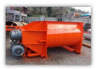
THE MIXER IS PROVIDING HOMOGENEOUS MIXING OF AGGREGATE. MOTOR POWER IS 2  $\times$  37 kw.HANDLE SYSTEM IS AS REPLACEABLE DESIGNED. BY THE PALLETS HANDLE - BY BASE WEAR PLATES AND BY ABRASION SHEET METAL HARDOX / ST 52 - A1 QUALITY MATERIAL IS USED.
