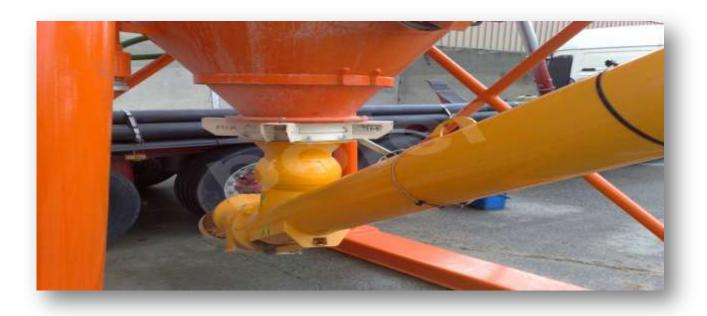
TAKES THE NEEDED CEMENT FOR MORTAR FROM THE SILO TO FEED THE WEIGHING CONVEYOR. WAM BRAND. 8'(\$\phi 219 \text{ mm}) MOTOR POWER IS 9,2 Kw. SILO CONNECTION POINT IS MOVABLE.
