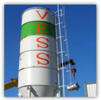
CEMENT STORAGE EQUIPMENT. BESIDES ARE WALKING STAIRS FOR EMERGENCIES. THE CAPACITY IS 75 TON AND REPLACEABLE CARTRIDGE FILTER IS PROVIDED. THERE IS ALSO 2 PIECES LEVEL MEASURING CENSOR PROVIDED AND SAFETY VALVE TO PREVENT OVERFILLING. TO DISCHARGE THE SILO INTO THE CEMENT FEEDING SCREW THERE IS A WAM BRAND VALVE. MANUFACTURED AS STEEL CONSTRUCTION USING 5/6 mm SHEET METAL.
