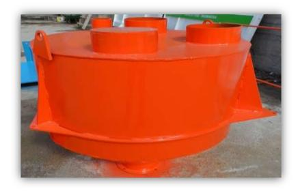
THIS DEVICE IS PROVIDING THE WEIGHING AND SENDING MATERIALS SUCH AS CEMENT – COLOR PIGMENT AND ADDITIVES TO THE MIXER. THE WEIGHING IS PROVIDED WITH 3 PIECES OF 500 Kg. LOADCELL. WAM BRAND ACTUATOR WITH VALVE AND MICRO SWITCH IS USED. **WATER**; WILL BE ADDED TO THE MORTAR VIA WEIGHING HOPPER OR DIGITAL WATER METER. THE CAPACITY OF ADDITIVE WEIGHING HOPPER IS 50 kg. COLOR PIGMENT WEIGHING HOPPER IS 100 kg.
