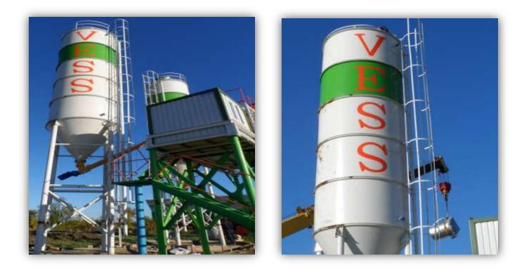
CEMENT STORAGE EQUIPMENT. BESIDES ARE WALKING STAIRS FOR EMERGENCIES. THE CAPACITY IS 75 TON AND REPLACEABLE CARTRIDGE FILTER IS PROVIDED. THERE IS ALSO 2 PIECES LEVEL MEASURING CENSOR PROVIDED AND SAFETY VALVE TO PREVENT OVERFILLING. TO DISCHARGE THE SILO INTO THE CEMENT FEEDING SCREW THERE IS A WAM BRAND VALVE. MANUFACTURED AS STEEL CONSTRUCTION USING 5 /6 mm. SHEET METAL.
