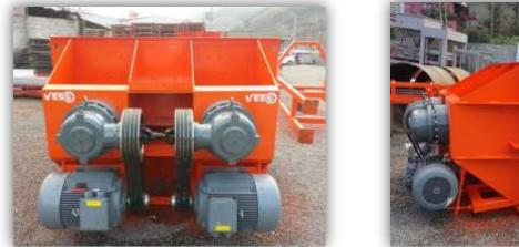
THE MIXER IS PROVIDING HOMOGENEOUS MIXING OF AGGREGATE. MOTOR POWER IS 2 x 45 kw. SLEEVE SYSTEM IS AS REPLACEABLE DESIGNED. BY THE PALLETS SLEEVE - BY BASE WEAR PLATES AND BY ABRASION SHEET METAL HARDOX / ST 52 - A1 QUALITY MATERIAL IS USED.
