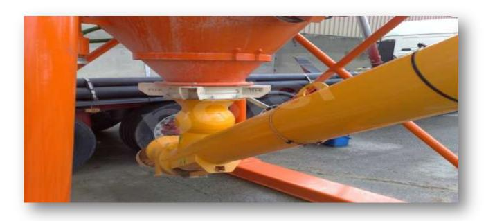
TAKES THE NEEDED CEMENT FOR MORTAR FROM THE SILO TO FEED THE WEIGHING CONVEYOR. WAM BRAND. 8'(\$\psi 219\text{ mm}\) MOTOR POWER IS 9,2 Kw. SILO CONNECTION POINT IS MOVABLE.
