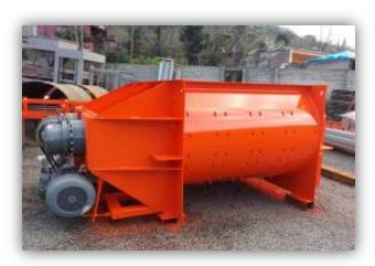
THE MIXER IS PROVIDING HOMOGENEOUS MIXING OF AGGREGATE. MOTOR POWER IS 2  $\times$  45 kw.HANDLE SYSTEM IS AS REPLACEABLE DESIGNED. BY THE PALLETS HANDLE - BY BASE WEAR PLATES AND BY ABRASION SHEET METAL HARDOX / ST 52 - A1 QUALITY MATERIAL IS USED.
