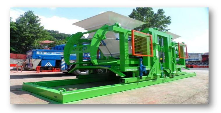
**MORTAR UNIT BASE PLATES: HARDOX 450**
