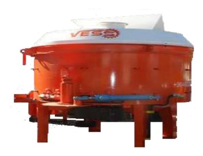
THE MIXER IS PROVIDING HOMOGENEOUS MIXING OF AGGREGATE. MOTOR POWER IS 15 kw. SLEEVE SYSTEM IS AS REPLACEABLE DESIGNED. BY THE PALLETS HANDLE - BY BASE WEAR PLATES AND BY ABRASION SHEET METAL HARDOX / ST 52 - A1 QUALITY MATERIAL IS USED.
