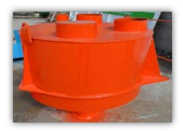
THIS DEVICE IS PROVIDING THE WEIGHING AND SENDING MATERIALS SUCH AS CEMENT – COLOR PIGMENT AND ADDITIVES TO THE MIXER. THE WEIGHING IS PROVIDED WITH 3 PIECES OF 1500 Kg. LOADCELL. WAM BRAND ACTUATOR WITH VALVE AND MICRO SWITCH IS USED. **WATER**; WILL BE ADDED TO THE MORTAR VIA WEIGHING HOPPER OR DIGITAL WATER METER. THE CAPACITY OF ADDITIVE WEIGHING HOPPER IS 200kg. COLOR PIGMENT WEIGHING HOPPER IS 200kg.
