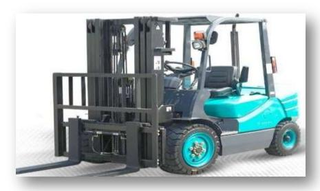
TRANSFERS THE PRODUCTS READY FOR SHIPMENT TO THE STOCKING AREA WHICH ARE ALREADY PACKED DIESEL – ISUZU MOTOR 3 TON CARRYING CAPACITY AND h; 4.20 MT LIFTING CAPABILITY.
