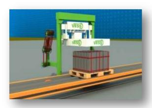
VERTICAL AND HORIZONTAL STRIPING EQUIPMENTS FOR THE PRODUCTS, STACKED ON THE EURO PALLET BY CONCRETE PRODUCT COLLECTING ROBOT. HAS THE FEATURE TO OPERATE FULLY AUTOMATIC.
