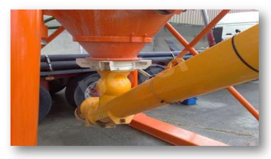
TAKES THE NEEDED CEMENT FOR MORTAR FROM THE SILO TO FEED THE WEIGHING CONVEYOR . WAM BRAND. 8'(\$\psi^2\$19 mm ) MOTOR POWER IS 9,2 Kw. SILO CONNECTION POINT IS MOVABLE.
