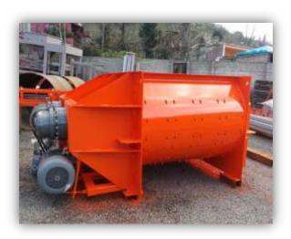
THE MIXER IS PROVIDING HOMOGENEOUS MIXING OF AGGREGATE. MOTOR POWER IS 2  $\times$  55 kw. SLEEVE SYSTEM IS AS REPLACEABLE DESIGNED. BY THE PALLETS SLEEVE - BY BASE WEAR PLATES AND BY ABRASION SHEET METAL HARDOX / ST 52 - A1 QUALITY MATERIAL IS USED.
