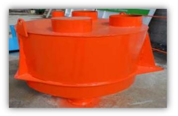
(08) – WEIGHING HOPPER (CEMENT / WATER /ADDITIVE / COLOR PIGMENT )
