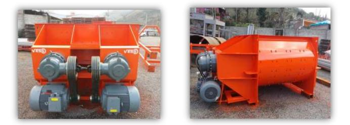
THE MIXER IS PROVIDING HOMOGENEOUS MIXING OF AGGREGATE. MOTOR POWER IS 2 x 90 kw. SLEEVE SYSTEM IS AS REPLACEABLE DESIGNED. BY THE PALLETS SLEEVE - BY BASE WEAR PLATES AND BY ABRASION SHEET METAL HARDOX / ST 52 - A1 QUALITY MATERIAL IS USED.
