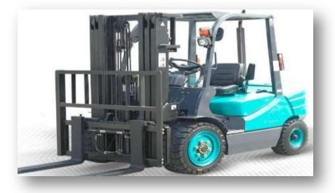
TRANSFERS THE PRODUCTS READY FOR SHIPMENT TO THE STOCKING AREA WHICH ARE ALREADY PACKED DIESEL – ISUZU MOTOR 3 TON CARRYING CAPACITY AND h; 4.20 MT LIFTING CAPABILITY.
