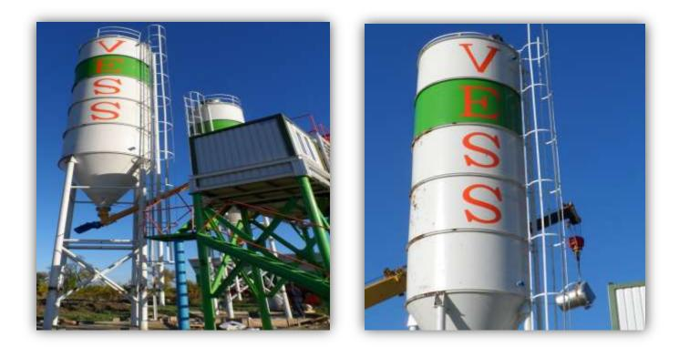
CEMENT STORAGE EQUIPMENT. BESIDES ARE WALKING STAIRS FOR EMERGENCIES. THE CAPACITY IS 100 TON AND REPLACEABLE CARTRIDGE FILTER IS PROVIDED. THERE IS ALSO 2 PIECES LEVEL MEASURING CENSOR PROVIDED AND SAFETY VALVE TO PREVENT OVERFILLING. TO DISCHARGE THE SILO INTO THE CEMENT FEEDING SCREW THERE IS A WAM BRAND VALVE. MANUFACTURED AS STEEL CONSTRUCTION USING 5 /6 mm. SHEET METAL.
