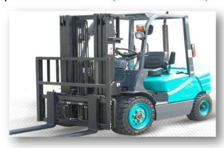
TRANSFERS THE PRODUCTS READY FOR SHIPMENT TO THE STOCKING AREA WHICH ARE ALREADY PACKED DIESEL – ISUZU MOTOR 3 TON CARRYING CAPACITY AND h; 4.20 mt LIFTING CAPABILITY.
