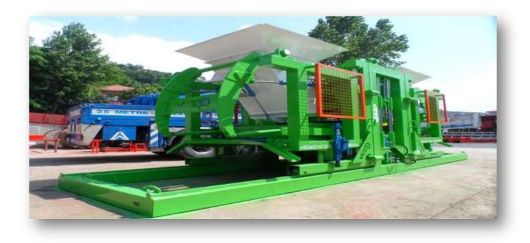
MORTAR UNIT BASE PLATES: HARDOX 450
