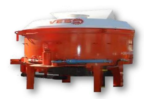
THE MIXER IS PROVIDING HOMOGENEOUS MIXING OF AGGREGATE. MOTOR POWER IS 22 kw. SLEEVE SYSTEM IS AS REPLACEABLE DESIGNED. BY THE PALLETS SLEEVE - BY BASE WEAR PLATES AND BY ABRASION SHEET METAL HARDOX / ST 52 - A1 QUALITY MATERIAL IS USED.
