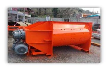
THE MIXER IS PROVIDING HOMOGENEOUS MIXING OF AGGREGATE. MOTOR POWER IS 2  $\times$  55 kw. SLEEVE SYSTEM IS AS REPLACEABLE DESIGNED. BY THE PALLETS SLEEVE - BY BASE WEAR PLATES AND BY ABRASION SHEET METAL HARDOX / ST 52 - A1 QUALITY MATERIAL IS USED.
