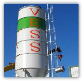
CEMENT STORAGE EQUIPMENT. BESIDES ARE WALKING STAIRS FOR EMERGENCIES. THE CAPACITY IS 100 TON AND REPLACEABLE CARTRIDGE FILTER IS PROVIDED. THERE IS ALSO 2 PIECES LEVEL MEASURING CENSOR PROVIDED AND SAFETY VALVE TO PREVENT OVERFILLING. TO DISCHARGE THE SILO INTO THE CEMENT FEEDING SCREW THERE IS A WAM BRAND VALVE. MANUFACTURED AS STEEL CONSTRUCTION USING 5/6 mm SHEET METAL.
