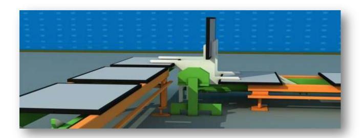
PROVIDES THAT THE PALLETS ARE TRANSFERRED TO THE PRESSING STATION AFTER REVERSING TO USE BOTH SIDES EQUALLY. DRIVEN BY 1,5 kw DRIVE CONTROLLED REDUCER.
