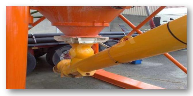
TAKES THE NEEDED CEMENT FOR MORTAR FROM THE SILO TO FEED THE WEIGHING CONVEYOR. WAM BRAND. 8'(\$\phi 219 \text{ mm}) MOTOR POWER IS 9,2 Kw. SILO CONNECTION POINT IS MOVABLE.
