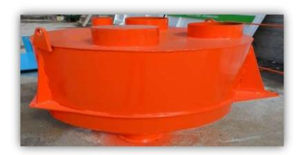
THIS DEVICE IS PROVIDING THE WEIGHING AND SENDING MATERIALS SUCH AS CEMENT – COLOR PIGMENT AND ADDITIVES TO THE MIXER. THE WEIGHING IS PROVIDED WITH 3 PIECES OF 1000 Kg. LOADCELL. WAM BRAND ACTUATOR WITH VALVE AND MICRO SWITCH IS USED. **WATER**; WILL BE ADDED TO THE MORTAR VIA WEIGHING HOPPER OR DIGITAL WATER METER. THE CAPACITY OF ADDITIVE WEIGHING HOPPER IS 100kg. COLOR PIGMENT WEIGHING HOPPER IS 150kg.
