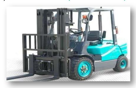
TRANSFERS THE PRODUCTS READY FOR SHIPMENT TO THE STOCKING AREA WHICH ARE ALREADY PACKED DIESEL – ISUZU MOTOR 3 TON CARRYING CAPACITY AND h; 4.20 mt LIFTING CAPABILITY.
