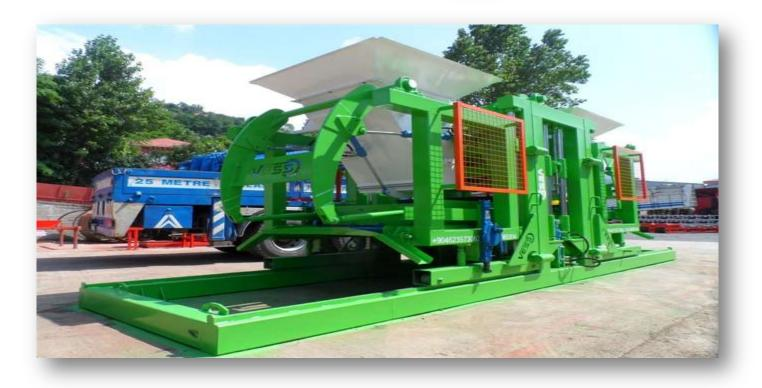
MORTAR UNIT BASE PLATES: HARDOX 450
