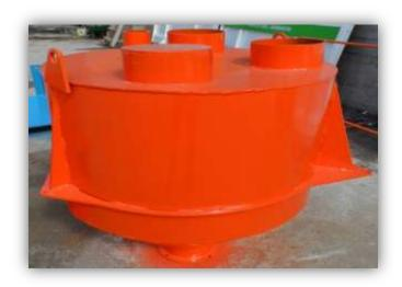
THIS DEVICE IS PROVIDING THE WEIGHING AND SENDING MATERIALS SUCH AS CEMENT – COLOR PIGMENT AND ADDITIVES TO THE MIXER. THE WEIGHING IS PROVIDED WITH 3 PIECES OF 500 Kg. LOADCELL. WAM BRAND ACTUATOR WITH VALVE AND MICRO SWITCH IS USED. **WATER**; WILL BE ADDED TO THE MORTAR VIA WEIGHING HOPPER OR DIGITAL WATER METER. THE CAPACITY OF ADDITIVE WEIGHING HOPPER IS 50kg. COLOR PIGMENT WEIGHING HOPPER IS 100kg.
