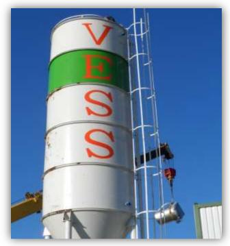
CEMENT STORAGE EQUIPMENT. BESIDES ARE WALKING STAIRS FOR EMERGENCIES. THE CAPACITY IS 75 TON AND REPLACEABLE CARTRIDGE FILTER IS PROVIDED. THERE IS ALSO 2 PIECES LEVEL MEASURING CENSOR PROVIDED AND SAFETY VALVE TO PREVENT OVERFILLING. TO DISCHARGE THE SILO INTO THE CEMENT FEEDING SCREW THERE IS A WAM BRAND VALVE. MANUFACTURED AS STEEL CONSTRUCTION USING 5 /6 mm. SHEET METAL.
