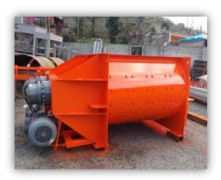
THE MIXER IS PROVIDING HOMOGENEOUS MIXING OF AGGREGATE. MOTOR POWER IS 2  $\times$  37 kw. HANDLE SYSTEM IS AS REPLACEABLE DESIGNED. BY THE PALLETS HANDLE - BY BASE WEAR PLATES AND BY ABRASION SHEET METAL HARDOX / ST 52 - A1 QUALITY MATERIAL IS USED.
