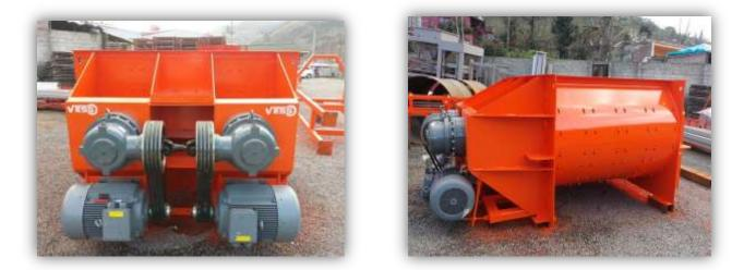
THE MIXER IS PROVIDING HOMOGENEOUS MIXING OF AGGREGATE. MOTOR POWER IS 2 x 45 kw. HANDLE SYSTEM IS AS REPLACEABLE DESIGNED. BY THE PALLETS HANDLE - BY BASE WEAR PLATES AND BY ABRASION SHEET METAL HARDOX / ST 52 - A1 QUALITY MATERIAL IS USED.
