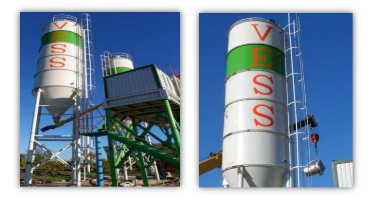
CEMENT STORAGE EQUIPMENT. BESIDES ARE WALKING STAIRS FOR EMERGENCIES. THE CAPACITY IS 100 TON AND REPLACEABLE CARTRIDGE FILTER IS PROVIDED. THERE IS ALSO 2 PIECES LEVEL MEASURING CENSOR PROVIDED AND SAFETY VALVE TO PREVENT OVERFILLING. TO DISCHARGE THE SILO INTO THE CEMENT FEEDING SCREW THERE IS A WAM BRAND VALVE. MANUFACTURED AS STEEL CONSTRUCTION USING 5 /6 mm. SHEET METAL.
