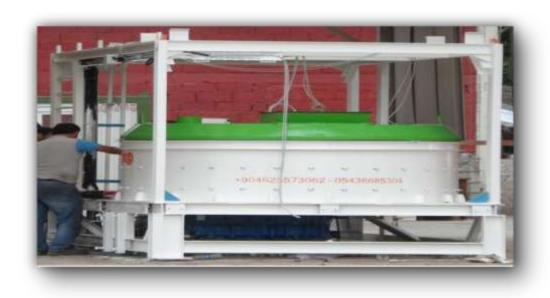
INSTALLATION PLATFORM FOR TWINSHAFT AND PAN TYPE MIXERS. MANUFACTURED USING NPU 120. BESIDES IS A WALKING PLATFORM FOR THE OPERATOR. IS DESIGNED FOR INSTALLATION OF 1 MIXER.
