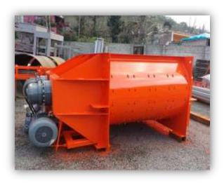
THE MIXER IS PROVIDING HOMOGENEOUS MIXING OF AGGREGATE. MOTOR POWER IS 2  $\times$  55 kw. HANDLE SYSTEM IS AS REPLACEABLE DESIGNED. BY THE PALLETS HANDLE - BY BASE WEAR PLATES AND BY ABRASION SHEET METAL HARDOX / ST 52 - A1 QUALITY MATERIAL IS USED.
