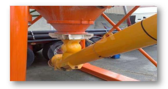
TAKES THE NEEDED CEMENT FOR MORTAR FROM THE SILO TO FEED THE WEIGHING CONVEYOR . WAM BRAND.  $8'(\emptyset 219 \text{ mm})$  MOTOR POWER IS 9,2 Kw. SILO CONNECTION POINT IS MOVABLE.
