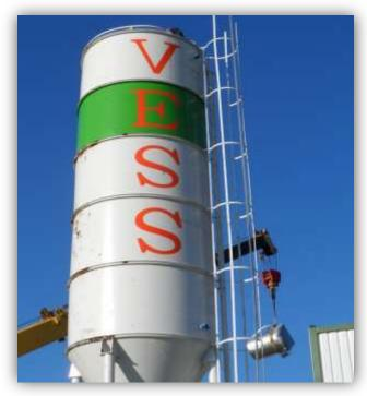
CEMENT STORAGE EQUIPMENT. BESIDES ARE WALKING STAIRS FOR EMERGENCIES. THE CAPACITY IS 100 TON AND REPLACEABLE CARTRIDGE FILTER IS PROVIDED. THERE IS ALSO 2 PIECES LEVEL MEASURING CENSOR PROVIDED AND SAFETY VALVE TO PREVENT OVERFILLING. TO DISCHARGE THE SILO INTO THE CEMENT FEEDING SCREW THERE IS A WAM BRAND VALVE. MANUFACTURED AS STEEL CONSTRUCTION USING 5 /6 mm. SHEET METAL.
