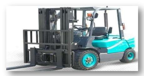
IS USED FOR THE TRANSPORTATION OF THE STACKED PALLETS TO THE DRYING ROOM AND TRANSFERS THE PALLETS TO THE REAR EMPTY PALLET UNLOADER ROBOT, COMING FROM THE DRYING ROOM.TRANSFERS ALSO THE PRODUCTS READY FOR SHIPMENT TO THE STOCKING AREA WHICH ARE ALREADY PACKED DIESEL – ISUZU MOTOR 3 TON CARRYING CAPACITY AND h; 4.20 MT LIFTING CAPABILITY.
