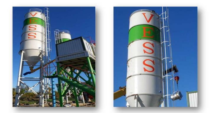
CEMENT STORAGE EQUIPMENT. BESIDES ARE WALKING STAIRS FOR EMERGENCIES. THE CAPACITY IS 200 TON AND REPLACEABLE CARTRIDGE FILTER IS PROVIDED. THERE IS ALSO 2 PIECES LEVEL MEASURING CENSOR PROVIDED AND SAFETY VALVE TO PREVENT OVERFILLING. TO DISCHARGE THE SILO INTO THE CEMENT FEEDING SCREW THERE IS A WAM BRAND VALVE. MANUFACTURED AS STEEL CONSTRUCTION USING 5/6 mm SHEET METAL.
