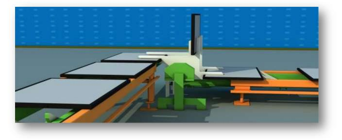
PROVIDES THAT THE PALLETS ARE TRANSFERRED TO THE PRESSING STATION AFTER REVERSING TO USE BOTH SIDES EQUALLY. DRIVEN BY 1,5 kw DRIVE CONTROLLED REDUCER.
