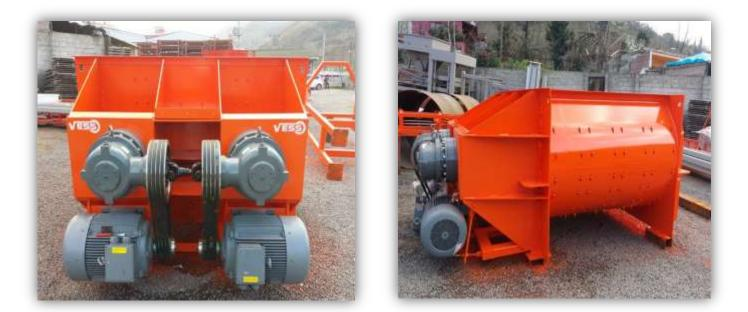
THE MIXER IS PROVIDING HOMOGENEOUS MIXING OF AGGREGATE. MOTOR POWER IS 2 x 90 kw.HANDLE SYSTEM IS AS REPLACEABLE DESIGNED. BY THE PALLETS HANDLE - BY BASE WEAR PLATES AND BY ABRASION SHEET METAL HARDOX / ST 52 - A1 QUALITY MATERIAL IS USED.
