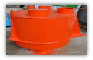
THIS DEVICE IS PROVIDING THE WEIGHING AND SENDING MATERIALS SUCH AS CEMENT – COLOR PIGMENT AND ADDITIVES TO THE MIXER. THE WEIGHING IS PROVIDED WITH 3 PIECES OF 2000 Kg. LOADCELL. WAM BRAND ACTUATOR WITH VALVE AND MICRO SWITCH IS USED. **WATER**; WILL BE ADDED TO THE MORTAR VIA WEIGHING HOPPER OR DIGITAL WATER METER. THE CAPACITY OF ADDITIVE WEIGHING HOPPER IS 400kg. COLOR PIGMENT WEIGHING HOPPER IS 300kg.
