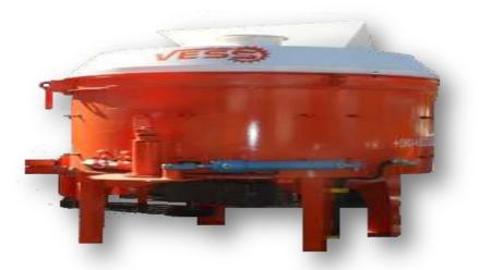
THE MIXER IS PROVIDING HOMOGENEOUS MIXING OF AGGREGATE. MOTOR POWER IS 22 kw. SLEEVE SYSTEM IS AS REPLACEABLE DESIGNED. BY THE PALLETS HANDLE - BY BASE WEAR PLATES AND BY ABRASION SHEET METAL HARDOX / ST 52 - A1 QUALITY MATERIAL IS USED.
