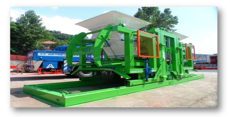
MORTAR UNIT BASE PLATES: HARDOX 450
