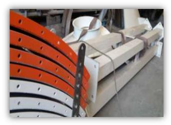
FOR EASY SHIPMENT; OPTIONALLY THE SILO CAN BE MANUFACTURED AS DEMOUNTED (BOLTED)
