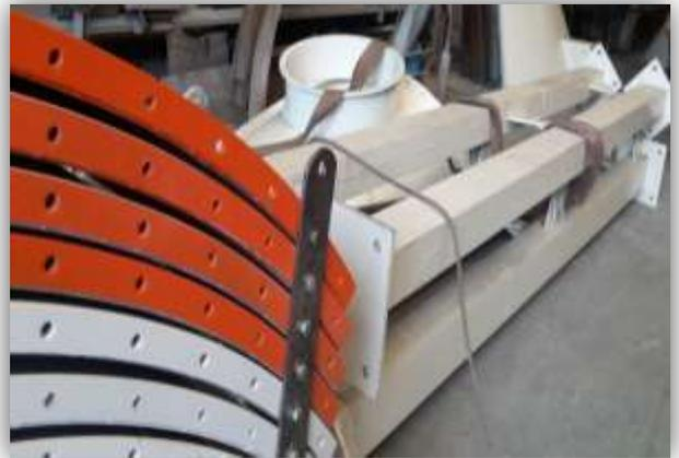
**FOR EASY SHIPMENT; OPTIONALLY THE SILO CAN BE MANUFACTURED AS DEMOUNTED ( BOLTED)**
