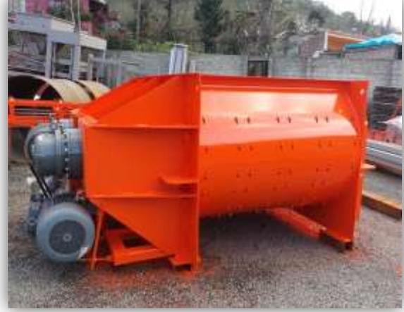
THE MIXER IS PROVIDING HOMOGENEOUS MIXING OF AGGREGATE. MOTOR POWER IS 2 x 90 kw. HANDLE SYSTEM IS AS REPLACEABLE DESIGNED. BY THE PALLET HANDLE - BY BASE WEAR PLATES AND BY ABRASION SHEET METAL HARDOX / ST 52 - A1 QUALITY MATERIAL IS USED.
