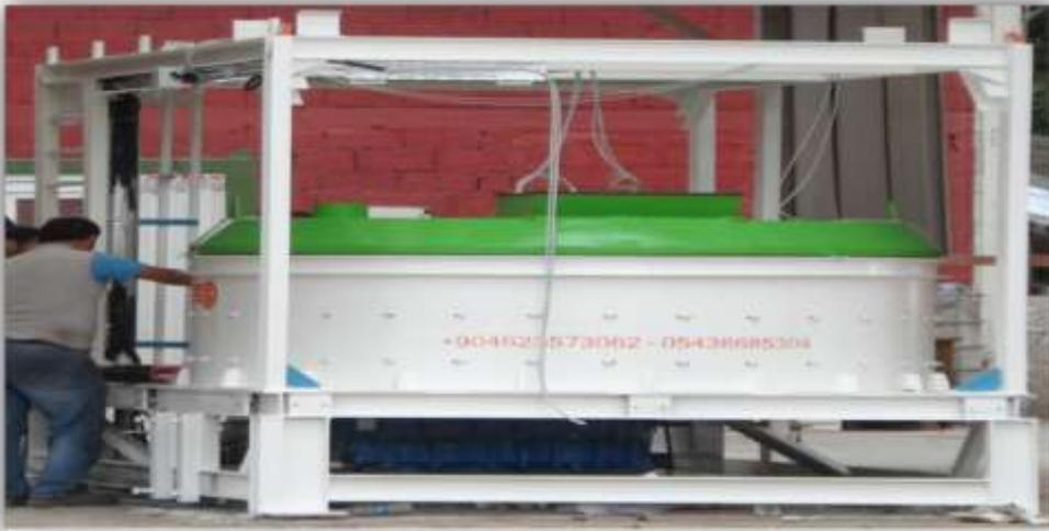
INSTALLATION PLATFORM FOR TWINSHAFT AND PAN TYPE MIXERS. MANUFACTURED USING NPU 120. BESIDES IS A WALKING PLATFORM FOR THE OPERATOR. IS DESIGNED FOR INSTALLATION OF 1 MIXER.
