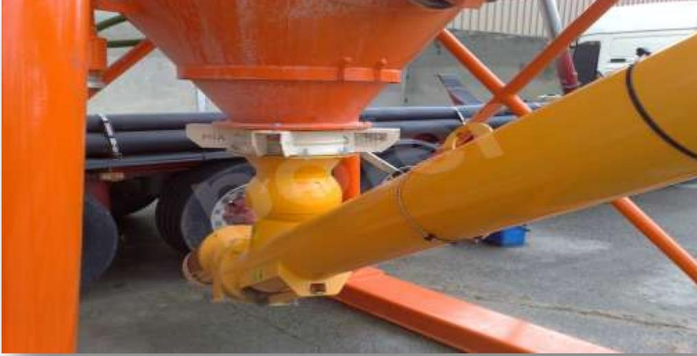
TAKES THE NEEDED CEMENT FOR MORTAR FROM THE SILO TO FEED THE WEIGHING CONVEYOR . WAM BRAND. 8'(Ø219 mm ) MOTOR POWER IS 9,2 Kw. SILO CONNECTION POINT IS MOVABLE.
