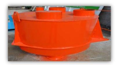
THIS DEVICE IS PROVIDING THE WEIGHING AND SENDING MATERIALS SUCH AS CEMENT – COLOR PIGMENT AND ADDITIVES TO THE MIXER. THE WEIGHING IS PROVIDED WITH 3 PIECES OF 500 Kg. LOADCELL. WAM BRAND ACTUATOR WITH VALVE AND MICRO SWITCH IS USED. **WATER**; WILL BE ADDED TO THE MORTAR VIA WEIGHING HOPPER OR DIGITAL WATER METER. THE CAPACITY OF ADDITIVE WEIGHING HOPPER IS 50kg. COLOR PIGMENT WEIGHING HOPPER IS 100kg.
