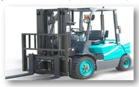
IS USED FOR THE TRANSPORTATION OF THE STACKED PALLETS TO THE DRYING ROOM AND TRANSFERS THE PALLETS TO THE REAR EMPTY PALLET UNLOADER ROBOT, COMING FROM THE DRYING ROOM.TRANSFERS ALSO THE PRODUCTS READY FOR SHIPMENT TO THE STOCKING AREA WHICH ARE ALREADY PACKED DIESEL – ISUZU MOTOR 3 TON CARRYING CAPACITY AND h; 4.20 MT LIFTING CAPABILITY.
