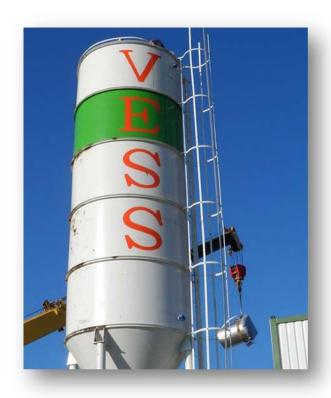
CEMENT STORAGE EQUIPMENT. BESIDES ARE WALKING STAIRS FOR EMERGENCIES. THE CAPACITY IS 200 TON AND REPLACEABLE CARTRIDGE FILTER IS PROVIDED. THERE IS ALSO 2 PIECES LEVEL MEASURING CENSOR PROVIDED AND SAFETY VALVE TO PREVENT OVERFILLING. TO DISCHARGE THE SILO INTO THE CEMENT FEEDING SCREW THERE IS A WAM BRAND VALVE. MANUFACTURED AS STEEL CONSTRUCTION USING 5/6 mm SHEET METAL.
