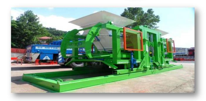
MORTAR UNIT BASE PLATES: HARDOX 450
