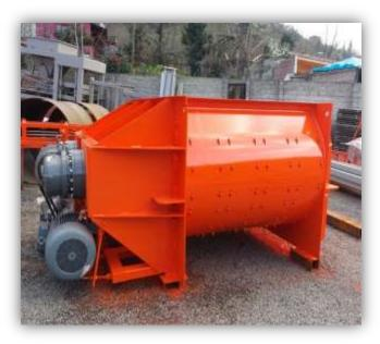
THE MIXER IS PROVIDING HOMOGENEOUS MIXING OF AGGREGATE. MOTOR POWER IS 2  $\times$  90 kw.HANDLE SYSTEM IS AS REPLACEABLE DESIGNED. BY THE PALLETS HANDLE - BY BASE WEAR PLATES AND BY ABRASION SHEET METAL HARDOX / ST 52 - A1 QUALITY MATERIAL IS USED.
