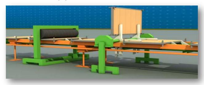
PROVIDES THAT THE PALLETS ARE TRANSFERRED TO THE PRESSING STATION AFTER REVERSING TO USE BOTH SIDES EQUALLY. DRIVEN BY 1,5 kw DRIVE CONTROLLED REDUCER.
