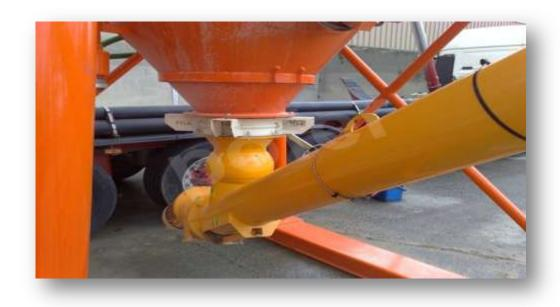
TAKES THE NEEDED CEMENT FOR MORTAR FROM THE SILO TO FEED THE WEIGHING CONVEYOR. WAM BRAND. 8'(\$\psi 219\text{ mm}\)) MOTOR POWER IS 9,2 Kw. SILO CONNECTION POINT IS MOVABLE.
