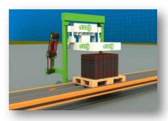
VERTICAL AND HORIZONTAL STRIPING EQUIPMENTS FOR THE PRODUCTS, STACKED ON THE EURO PALLET BY CONCRETE PRODUCT COLLECTING ROBOT. HAS THE FEATURE TO OPERATE FULLY AUTOMATIC.
