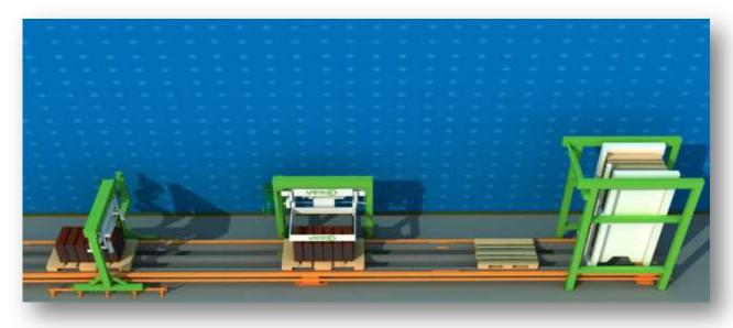
SEPARATE THE PALLETS NEEDED FOR SHIPPING ONE BY ONE AND SEND TO THE PACKAGING STATION.
