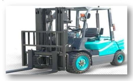
IS USED FOR THE TRANSPORTATION OF THE STACKED PALLETS TO THE DRYING ROOM AND TRANSFERS THE PALLETS TO THE REAR EMPTY PALLET UNLOADER ROBOT, COMING FROM THE DRYING ROOM.TRANSFERS ALSO THE PRODUCTS READY FOR SHIPMENT TO THE STOCKING AREA WHICH ARE ALREADY PACKED DIESEL – ISUZU MOTOR 3 TON CARRYING CAPACITY AND h; 4.20 MT LIFTING CAPABILITY.
