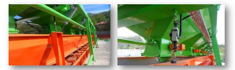
**WEIGHING COMPARTMENT:** THIS IS THE COMPARTMENT WHERE IS THE AGGREGA COMING FROM THE HOPPER DISCHARGE COVER STOCKED . USED 5 MM SHEET METAL. DESIGNED BENDING TO INCREASE THE STRENGTH. INCLUDING FLOW CONTROL PANEL TO EXTEND THE BAND TIRES LIFE AND REDUCE THE LOAD ON THE BAND. THE WEIGHING COMPARTMENT IS COMPLETELY REMOVABLE AND SEPARABLE.
