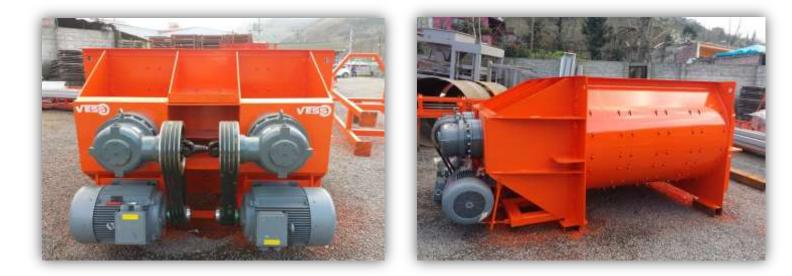
THE EQUIPMENT IS PROVIDING HOMOGENEOUS MIXING OF DOSAGED AGGREGATE.
