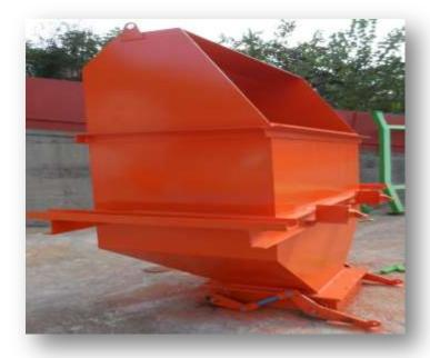
THE PLACE WHERE THE READY WEIGHED AGREGAS HOLD AS A RESERVED. WITH THIS, DOSAGED AGREGA STAYS HERE WHILE MIXING OPERATION AND SAVE THE TIME WHILE LOADING AGAIN. AGRFGA HOLDING HOPPFR MANUFACTURED 5 mm SHEET METAL AND NPL 70 BRACKET. UNLOADING FUNNELS IS 5 mm. THICK METAL SHEET IS USED. BY THE SMOOTH SURFACES ARE ALSO 3mm. REPLACEABLE WEAR PLATE. COVERS ARE MANUFACTURED USING 5 mm METAL SHEET, THE FLOWING IS STRENGTHENED WITH THE PNEUMATIC SYSTEM ON THE HOPPER.
