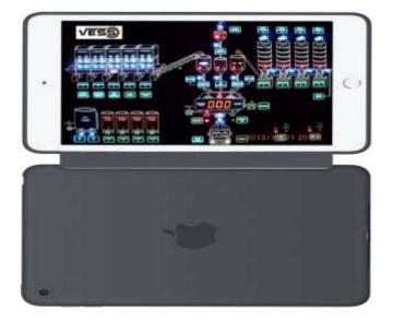
ALUMINATION AND CALIBRATION PROCEDURES CAN BE DISPLAYED ON THE OPERATOR PANEL; PROCESS, PRODUCTION AND ERROR MESSAGES.
