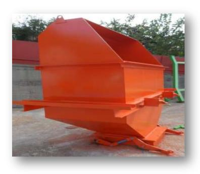
THE PLACE WHERE THE READY WEIGHED AGREGAS HOLD AS A RESERVED. WITH THIS, DOSAGED AGREGA STAYS HERE WHILE MIXING OPERATION AND SAVE THE TIME WHILE LOADING AGAIN. AGREGA HOLDING **HOPPER** MANUFACTURED 5 mm SHEET METAL AND NPL 70 BRACKET. UNLOADING FUNNELS IS 5 mm. THICK METAL SHEET IS USED. BY THE SMOOTH SURFACES ARE ALSO 3mm. REPLACEABLE WEAR PLATE. COVERS ARE MANUFACTURED USING 5 METAL SHEET, THE FLOWING IS STRENGTHENED WITH THE PNEUMATIC SYSTEM ON THE HOPPER.
