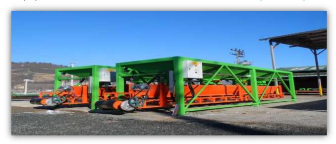
THIS CONVEYOR ALLOWS THE WEIGHING OF THE AGGREGATE IN THE HOPPER AND AFTER WEIGHING TRANSFERS THE AGGREGATE TO THE TRANSFER BAND. POSITIONED JUST BELOW THE AGGREGA HOPPER. IT CONTAINS **5 COMPONENT** WEIGHING COMPARTMENT, CHASSIS, CONVEYOR TIRE, ROLLS WEIGHING SYSTEM AND MOTOR REDUCTOR GROUP.
