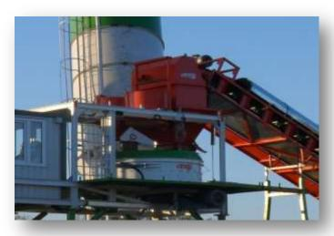
PISTON TO WORK IN LINES WITHOUT PRESSURE. WATER: THIS DEVICE IS PROVIDING THE NEEDED WATER TO THE MIXER. WEIGHING CAPACITY IS **250 KG**. THE WEIGHING IS PROVIDED WITH **3 PIECES OF 500 Kg**. LOADCELL. WAM BRAND ACTUATOR WITH VALVE AND MICRO SWITCH IS USED. THERE ARE TWO LINES TO TAKE WATER IN THE SYSTEM. POSSIBLE TO USE 2. LINE FOR SENSITIVE HUMIDITY RATIO.
