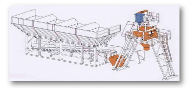
OPTIONALLY, AGREGA CAN TRANSFER TO MIXER ALSO WITH BUCKET SYSTEM.
