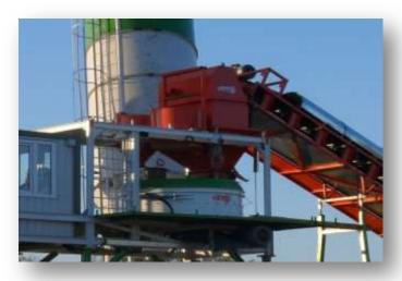
PISTON TO WORK IN LINES WITHOUT PRESSURE. WATER: THIS DEVICE IS PROVIDING THE NEEDED WATER TO THE MIXER. WEIGHING CAPACITY IS 400 KG. THE WEIGHING IS PROVIDED WITH 3 PIECES OF 500 Kg. LOADCELL. WAM BRAND ACTUATOR WITH VALVE AND MICRO SWITCH IS USED. THERE ARE TWO LINES TO TAKE WATER IN THE SYSTEM. POSSIBLE TO USE 2. LINE FOR SENSITIVE HUMIDITY RATIO.
