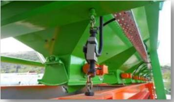
WEIGHING COMPARTMENT: THIS IS THE COMPARTMENT WHERE IS THE AGGREGA COMING FROM THE HOPPER DISCHARGE COVER STOCKED. USED 5 MM SHEET METAL. DESIGNED BENDING TO INCREASE THE STRENGTH. INCLUDING FLOW CONTROL PANEL TO EXTEND THE BAND TIRES LIFE AND REDUCE THE LOAD ON THE BAND. THE WEIGHING COMPARTMENT IS COMPLETELY REMOVABLE AND SEPARABLE.
