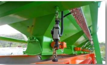
**WEIGHING COMPARTMENT:** THIS IS THE COMPARTMENT WHERE IS THE AGGREGA COMING FROM THE HOPPER DISCHARGE COVER STOCKED. DESIGNED BENDING TO INCREASE THE STRENGTH. INCLUDING FLOW CONTROL PANEL TO EXTEND THE BAND TIRES LIFE AND REDUCE THE LOAD ON THE BAND. THE WEIGHING COMPARTMENT IS COMPLETELY REMOVABLE AND SEPARABLE.
