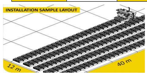
NOT: PRODUCTION AREA PLACEMENT, MANUAL MACHINES: FIELD SPREADING, MANUAL MACHINES LAYING WITH 5 cm GAP IN ORDER TO FORWARD, SIDEWARDS WITH 35 cm GAP. AUTOMATIC MACHINES: LAYING WITH IN ORDER TO FORWARD 20 cm GAP, SIDEWARDS WITH 35 cm. FOR THE MANUAL MACHINES RECOMMENDED CONCRETE AREA IS MIN 12x40 METER.
