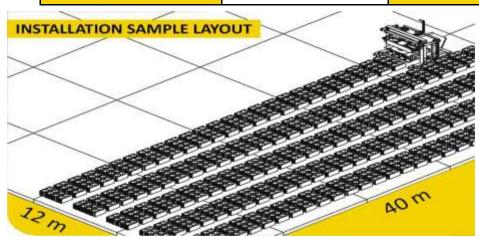
NOT: PRODUCTION AREA PLACEMENT, MANUAL MACHINES: LAYING WITH 5 cm GAP IN ORDER TO FORWARD, SIDEWARDS WITH 35 cm GAP. AUTOMATIC MACHINES LAYING WITH IN ORDER TO FORWARD 20 cm GAP, SIDEWARDS WITH 35 cm. FOR THE MANUAL MACHINES RECOMMENDED CONCRETE AREA IS MIN 12x40 METER.
