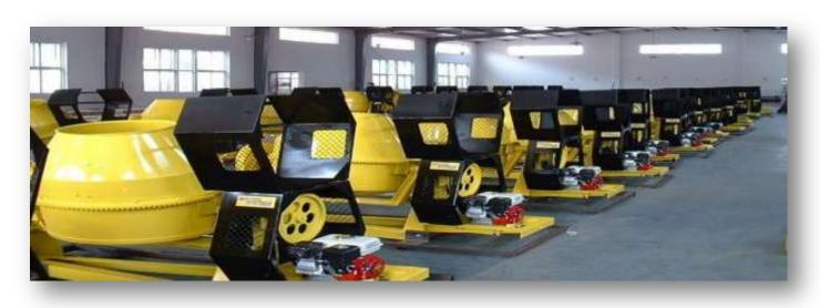
THE EQUIPMENT TO PREPARE MIXTURE FOR THE PRODUCT TO BE PRESSED. 380-400 It CAPACITY. CHANGEABLE GEAR EXIST. THERE IS A TAMBOUR BASE REINFORCED WITH STEEL BEAM. PROTECT WITH SAFE ELECTRICAL INSULATION. INNER HANDLES MAKE HOMOGENEOUS MIXTURE. UPPER AND LOWER PART OF TAMBUR CAN BE CHANGED SEPERATELY. MIXER DRIVE AND PULLEY CONCRETE BEARINGS PRODUCED BY QUALITY BEARINGS. EASY TO DISCHARGE WITH CONIC TAMBOUR. MIXER DOES NOT NEED MAINTENANCE.
