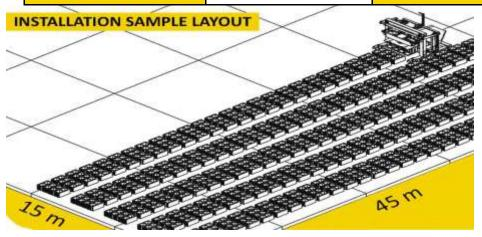
NOT: PRODUCTION AREA PLACEMENT, MANUAL MACHINES: LAYING WITH 5 cm GAP IN ORDER TO FORWARD, SIDEWARDS WITH 35 cm GAP. AUTOMATIC MACHINES THE MACHINE LAYING WITH IN ORDER TO FORWARD GAP 20 cm AND ALSO OPERATES TO NEAR SIDE 35 cm. FOR THE MANUAL MACHINES RECOMMENDED CONCRETE AREA IS MIN 15x45 METER.
