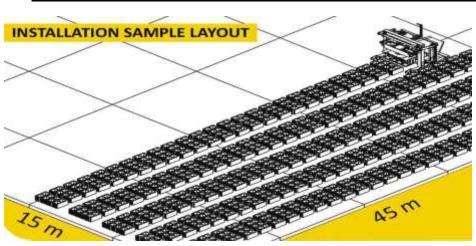
NOT: PRODUCTION AREA PLACEMENT, MANUAL MACHINES: THE MACHINE LAYING WITH 5 cm GAP IN ORDER TO FORWARD, SIDEWARDS WITH 35 cm GAP.AUTOMATIC MACHINES THE MACHINE LAYING WITH IN ORDER TO FORWARD 20 cm GAP,SIDEWARDS WITH 35 cm. FOR THE MANUAL MACHINES RECOMMENDED CONCRETE AREA IS MIN 15x45 METER.
