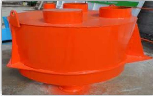
CET EQUIPEMENT PERMET DE PESER ET D'ENVOYER AU MALAXEUR (MALAXEUR) LES AGREGATS COMME CIMENT ET LES COLORANTS. AVEC **3 SORTIS DE 1.000 Kg** POUR LE DECHARGEMENT DES AGREGATS PESÉ PAR LE LOADCELL. LES EQUIPEMENTS COMME LE SOUPAPE ET LE MICRO INTERRUPTEUR DE LA MARQUE WAM EST UTILISÉ. L'AJOUT D'EAU AU MORTIER POUR LE MELANGE SE FAIT A PARTIR D'UN RESERVOIR D'EAU NUMÉRIQUE(LOADCELL). **100 Kg DE CAPACITE** POUR RESERVOIR D'AJOUT DES AGREGATS ET **150 Kg** POUR LA RESERVOIR DE COLORATION.
