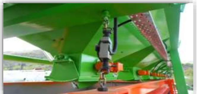
**(03) CONVOYEUR A BANDE (11.5m x 0.50m x 8mm) (MOUVEMENT DE GAUCHE-DROITE)**
