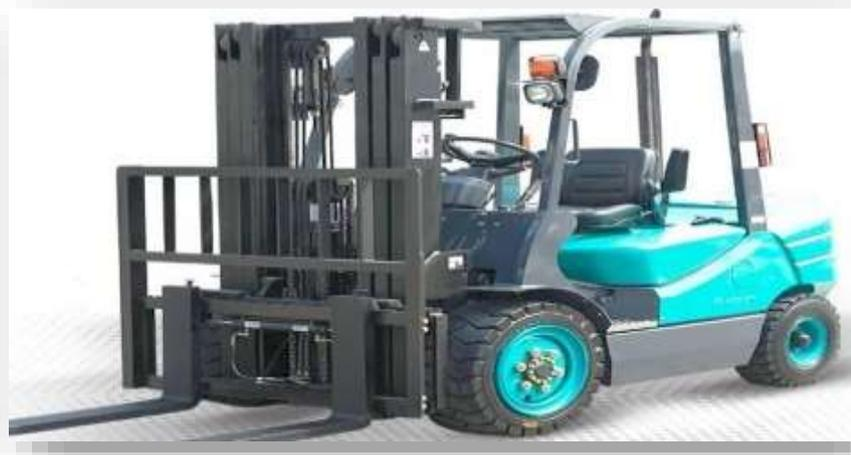
LA MACHINE A CHARIOT D'ÉLEVEUR ISUZU DE MARQUE ZAPONAISE. PERMET DE TRANSPORTER LES PRODUITS FINIS EMPILER PAR LE SYSTEME DE ROBOTAGE A LEUR LIEU DE SECHASSAGE OU DE STOCKAGE. ELLE PERMET DE DEPLACER AUSSI LES PALETTES VIDE VERS LE SYSTEME ROBOTIQUE DE DEPILLAGE. ELLE A UN MOTOR DIESEL AVEC UNE CAPACITE DE SOULEVAGE DE 3 TONNES ET H: 4,20m.
