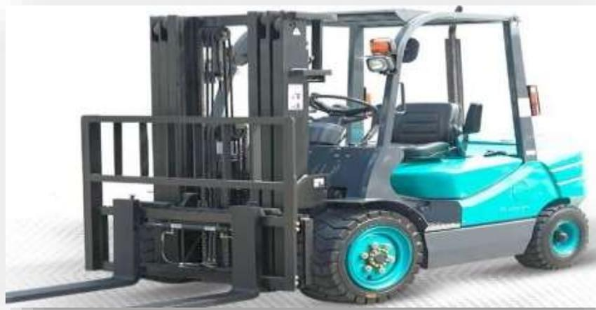
LA MACHINE A CHARIOT D’ELEVEUR ISUZU DE MARQUE ZAPONAISE. PERMET DE TRANSPORTER LES PRODUITS FINIS EMPILER PAR LE SYSTEME DE ROBOTAGE A LEUR LIEU DE SECHESSE OU DE STOCKAGE. ELLE PERMET DE DEPLACER AUSSI LES PALETTES VIDE VERS LE SYSTEME ROBOTIQUE DE DEPILAGE. ELLE A UN MOTOR DIESEL AVEC UNE CAPACITE DE SOULEVAGE DE 3 TONNES ET H:4,20m.
