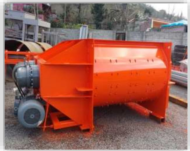
LE MALAXEUR TWINSHAFT MELANGE LES AGREGATS DE FAÇONS HOMOGENE. LA PUISSANCE DE CES MOTEURS **2 x 90 kw**. LE SYSTÈME DE MANIVELLE EST REMPLAÇABLE. PALETTES DES MANIVELLES ET LES PLAQUES D'USURE SONT FAIT AVEC DU **HARDOX /ST 52-A1**, UN MATERIEL DE QUALITÉ UTILISE POUR LEURS FABRICATIONS.
