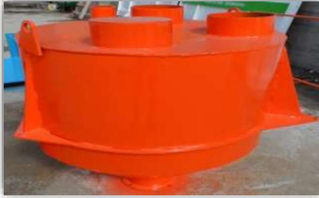
CET EQUIPEMENT PERMET DE PESER ET D'ENVOYER AU MALAXEUR (MALAXEUR) LES AGREGATS COMME CIMENT ET LES COLORANTS. AVEC **3 SORTIS DE 2.000Kg** POUR LE DECHARGEMENT DES AGREGATS PESÉ PAR LE LOADCELL. LES EQUIPEMENTS COMME LE SOUPEPE ET LE MICRO INTERRUPTEUR DE LA MARQUE WAM EST UTILISÉ. L'AJOUT D'EAU AU MORTIER POUR LE MELANGE SE FAIT A PARTIR D'UN RESERVOIR D'EAU NUMÉRIQUE(LOADCELL). **400Kg DE CAPACITE** POUR RESERVOIR D'AJOUT DES AGREGATS ET **300Kg** POUR LA RESERVOIR DE COLORATION.
