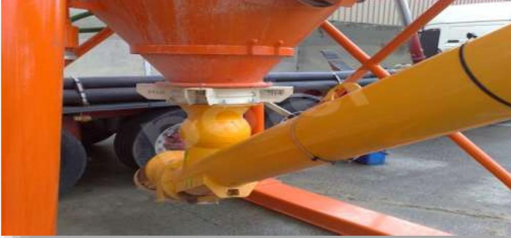
C'EST L'EQUIPEMENT QUI TRANSFERE LE CIMENT NECESSAIRE DU MORTIER AU SYSTEME DE PESAGE. ELLE EST DE LA **MARQUE WAM 8'' ( Ø219 mm )** PUISSANCE DU MOTEUR EST **9.2 Kw**. LE POINT DE LIAISONS DU SILO EST MOUVABLE.
