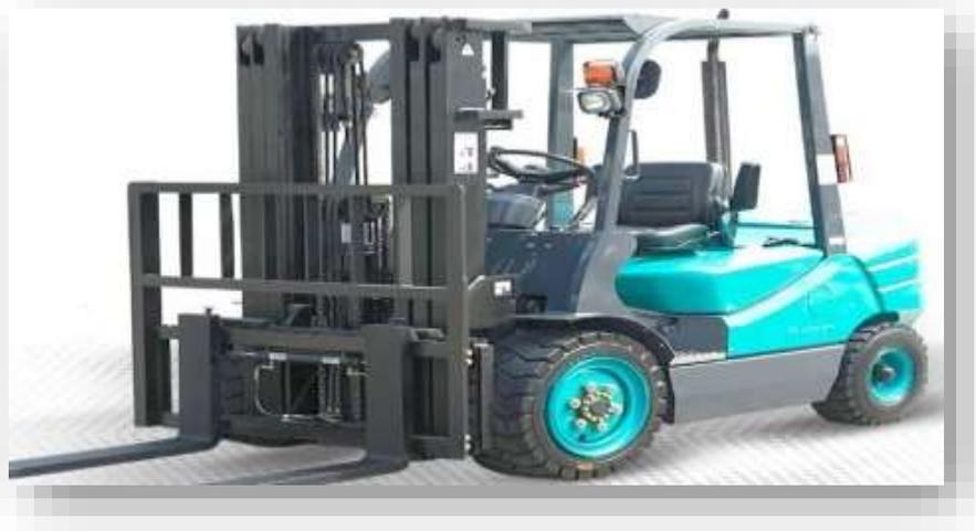
LA MACHINE A CHARIOT D’ELEVEUR ISUZU DE MARQUE ZAPONAISE. PERMET DE TRANSPORTER LES PRODUITS FINIS EMPILER PAR LE SYSTEME DE ROBOTAGE A LEUR LIEU DE SECHESSEGE OU DE STOCKAGE. ELLE PERMET DE DEPLACER AUSSI LES PALETTES VIDE VERS LE SYSTEME ROBOTIQUE DE DEPILAGE. ELLE A UN MOTOR DIESEL AVEC UNE CAPACITE DE SOULEVAGE DE 3 TONNES ET H: 4,20m.
